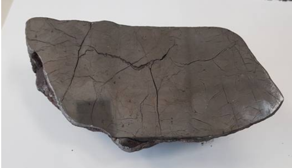
Photo 3 hand specimen of massive sulphide from Disko, large interlocking nickel-copper PGE rich crystals.
